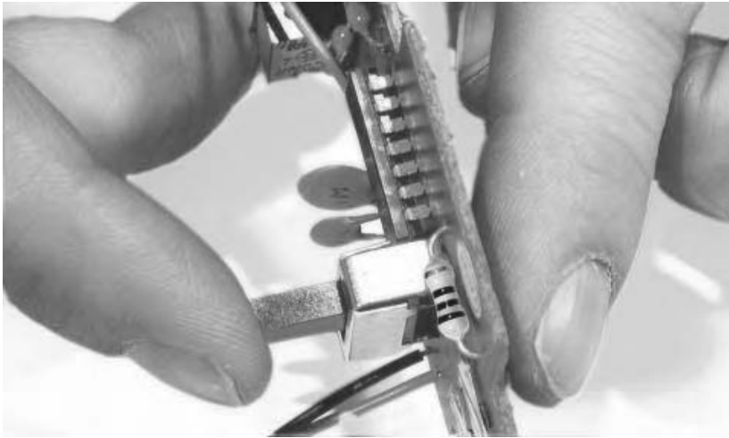
Figure 12.8 Finding the clock resistor (finger on right).
