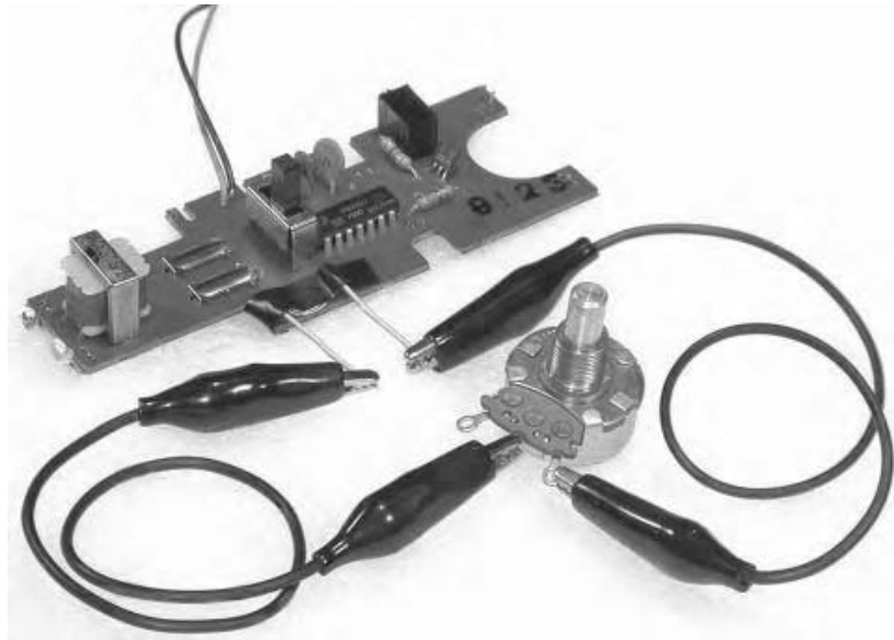
Figure 13.7 Pot substitute for a clock resistor.
