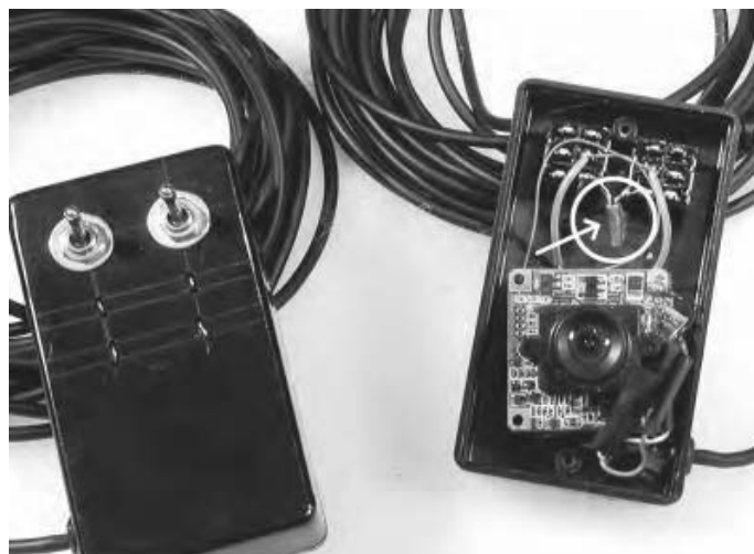
Figure 25.1 Camera board with switch for disconnecting crystal (circled, right) and electrodes for tickling clock frequency (left, visible below switches).
