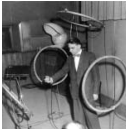
Pierre Henry, pupitre d'espace , a device utilizing induction coils, built by Jacques Poullin in 1951 at Pierre Schaeffer’s suggestion.
